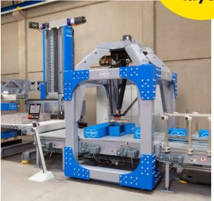
**Load capacity** Layer weight up to 150 kg
