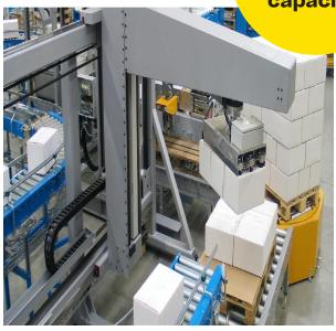
**Cycle capacity** Up to 4 layers / minute
