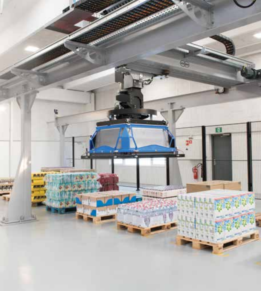
Körber's Layer Picker is the industry standard and leading technology for both de-palletizing and pallet-to-pallet picking.
