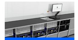
As each operation is unique and faces unique challenges, Körber specialists analyze each process and design the best way of working around the Attabotics port. Options include putt-walls operated by pick-to-light, automated empty cartons supply and conveying picked cartons to packing, shipping or other warehouse areas.
