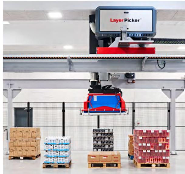
Components: Layer picker, gantry robot, palletbuffer, pallet transport, WCS software, stretchwrap and labelling, defoil and strapex.
