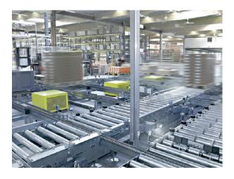
surrounding, circular conveyor system. It acts as a buffer zone, as well as a sequencing module for three picking stations in the shipping department; there, order picking takes place guided by K.Motion PMS-W. With confirmation of the picking orders, the conveyor system removes the partial pallets to the high-bay warehouse. At the same time, empty pallets are fed to an automatic pallet stacker.
