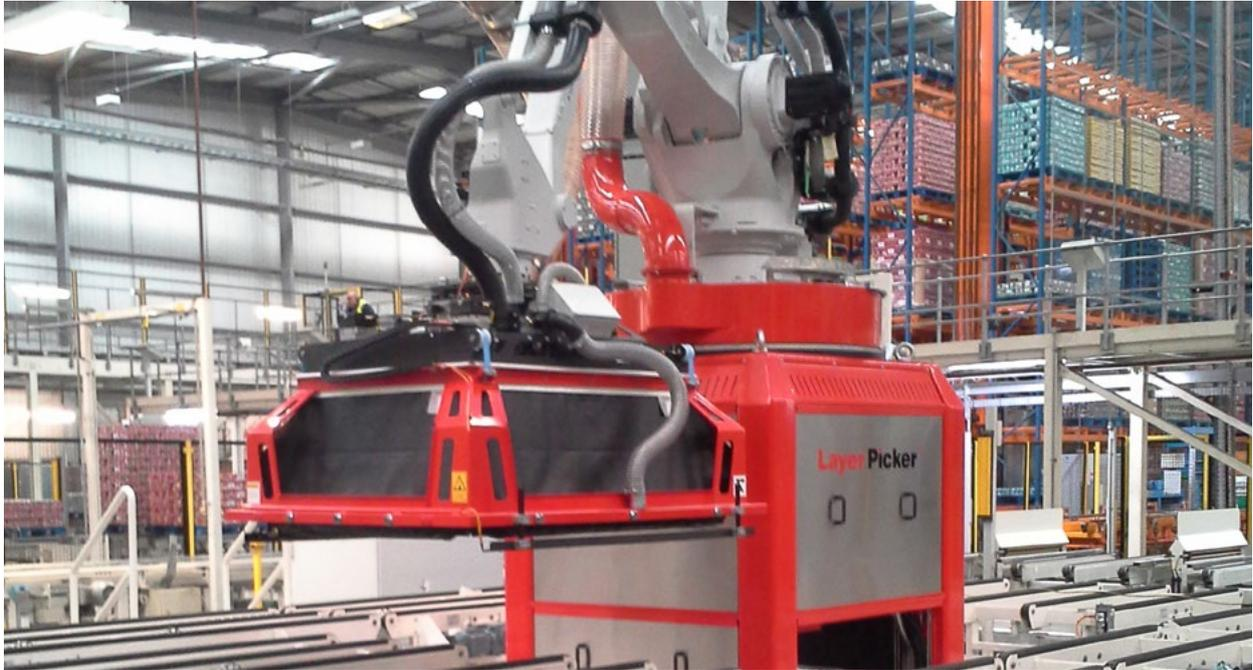
**Kraft Heinz wanted a significant increase in the amount of pallet layers being picked automatically without making changes in the existing product configuration. This was achieved with the installation of a K.Handle Layer Picker® Flex-R from Körber.**
