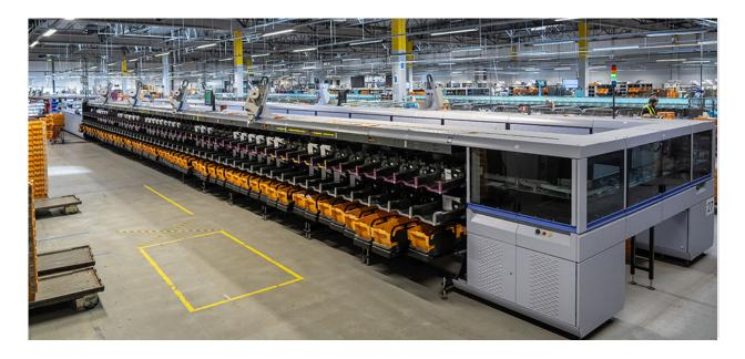
Within one year, Körber modernized and updated PostNord Denmark's mail sorting equipment. The project encompassed moving machines from Frederica to Taastrup, replacing machine control hard- and software, and upgrading the reading/coding system. This technology and generation mix integration was implemented during continued operation and adhered to the strict timeline.
