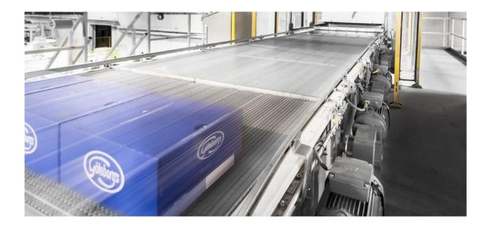
Netto decided to invest in a complete upgrade of the K.Handle Layer Picker® heads, stripper and descrambler units of their three Layer Pickers, after nine years of operating the facility 24/7, 6 days per week. After the upgrade it was possible to cut the regular working week from 6 to 5 days while increasing capacity at the same time.
