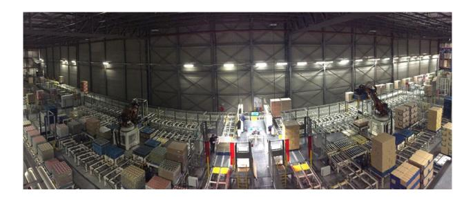
At the distribution center in Utrecht, the objective was once again to achieve intelligent material flow control for storage and retrieval, picking, and crossdocking. To attain intelligent, automated layer picking, layer picking robots from Körber were chosen. The cooperation between Kuehne + Nagel and Körber has been a unique one, characterized by a long and close history and a continuous dialogue throughout and after projects, with benefits for both companies.
