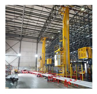
A loop with conveyors in front of the high bay and expedition docks guarantees the fine sequencing of the pallets to be loaded in the trucks, as well as an additional buffer.
